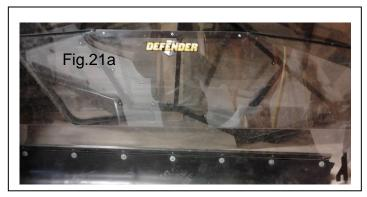
xx) With dump box open, re-install rear panel with (4) ½"-20 x 0.5"L hex screw & seal washers as shown. Fasten the top of the panel to the roof using (2) ½"-20 x 0.5"L hex screw & seal washers as well.
